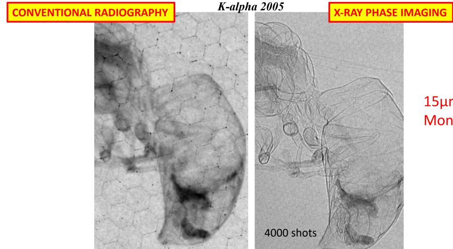
15µm X-ray source size Monochromatic X-rays
